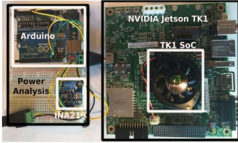
Fig. 5. Experimental setup for power measurement of TK1 board including, INA219 power monitor sensor, Arduino Uno microcontroller and TK1 CPU-GPU boards.
